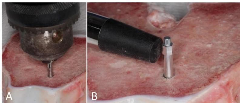
**Figure 2.** Measurement of insertion torque with a precision digital torque meter (A). Measurement of implant stability with resonance frequency analysis (B).
