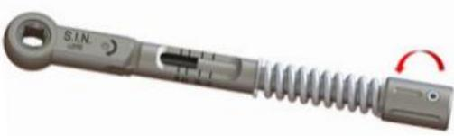
2. After loosening the drum, remove the body and the head from the torque wrench.
