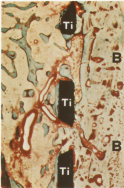
Fig. 9a Cylindrical implant which has been fully stressed for 12 months. As in Fig. 8, normal bone (B) has formed on the rough surface of the implant (Ti) and has remained in immediate contact despite the loads to which it has been subjected. (6 x).
